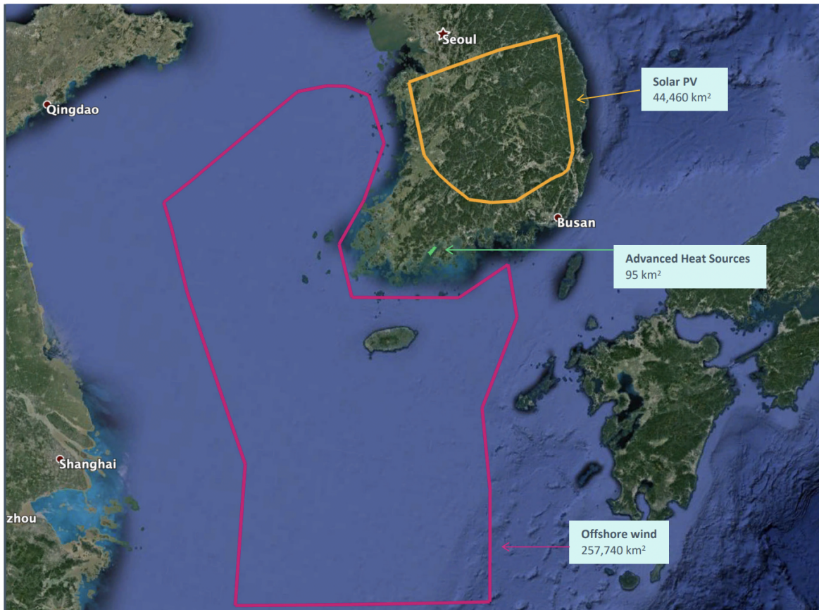
Each colored outline represents the total area that would be required for the siting of each type of resource if it were to be the only one used to generate enough hydrogen to replace current oil consumption in South Korea.
